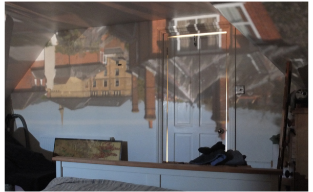
Camera obscura set up in the author’s bedroom (the photo was over exposed to brighten the image)
